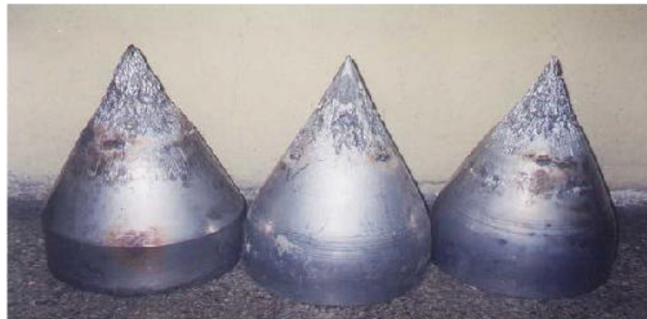
Figure 2 Severely worn Pelton needles.
