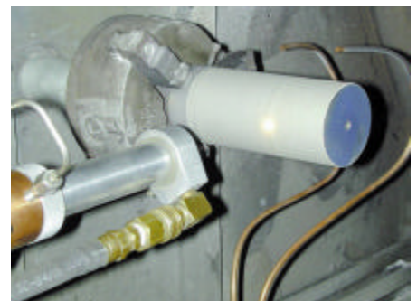
Figure 1 Experimental high-pressure HVOF device. Due to its low temperature the spray stream is barely visible.
