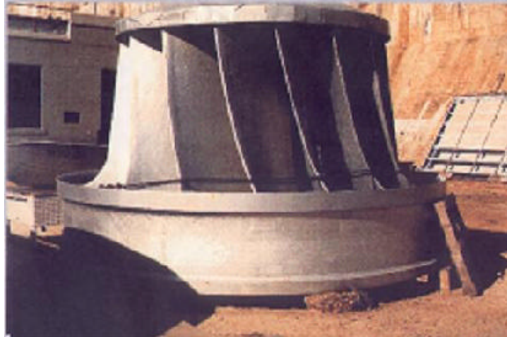
Figure 1 New turbine runner for Salal Station
