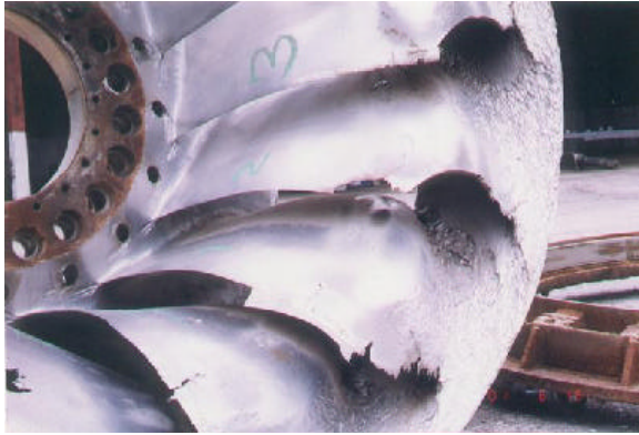
Figure 3 Severe erosion on Francis Turbine runner
