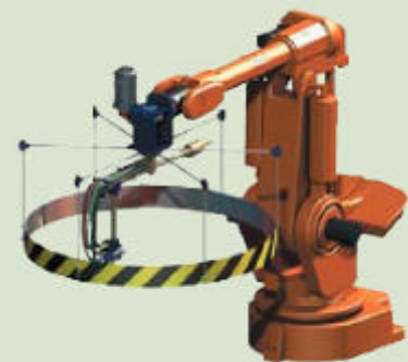
CAD drawing of the Rota DJ, an HVOF gun, fixed to a rotating fixture for coating internal surfaces.
