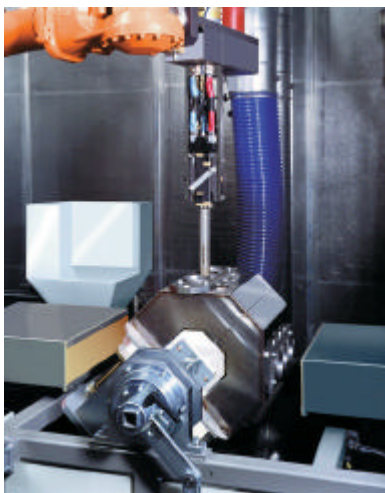
Plasma spraying a coating to the bore of an automotive lightweight cylinder block. The rotating extension is fed into the bore and the block remains stationary. ( photo by courtesy of Sulzer Metco Limited)
